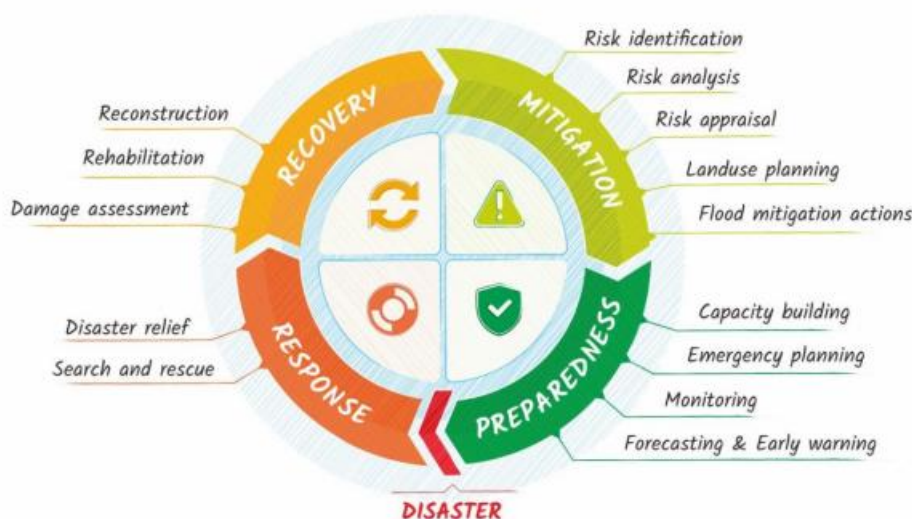
Figure IV-5 Key Flood Management Cycle Components (Reference ADB Practical Guide To Integrated Flood Risk Management (IFRM) 2022)
